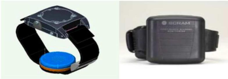
Figure 1: Alcohol Biosensor Devices: The WrisTAS (left) and the SCRAM (right).
